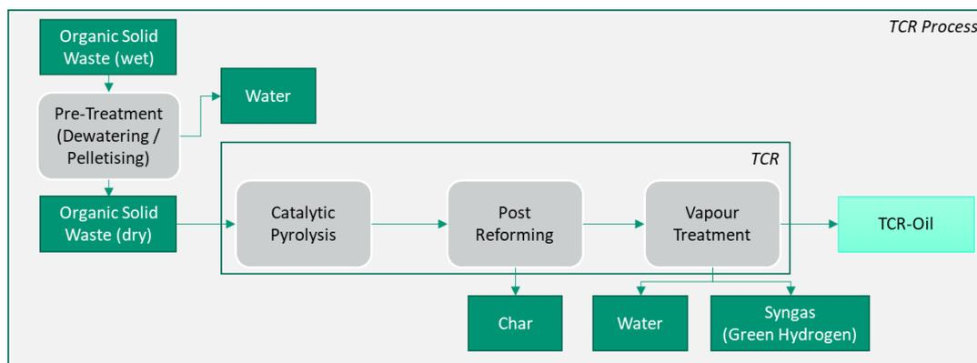
**Figure 2:** Thermo-Catalytic Reforming TCR®: A Platform Technology to use residues and to produce sustainable and storable energy carriers. [3]
