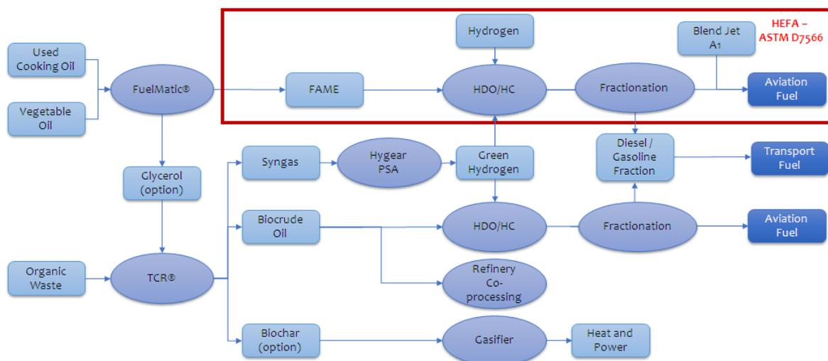
**Figure 3:** Process flow diagram.
